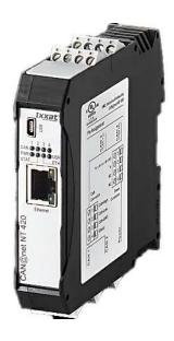
The Ixxat CAN@net NT 420 is a multifunctional gateway, bridging CAN and Ethernet networks for remote access and enhanced reliability. It features four CAN channels, thereof two CAN FD capable, and supports long-distance communication, with several message processing and cloud connection functionalities. For more efficient network management.
