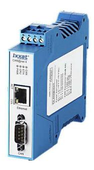
The CAN@net II/Generic with one CAN channel and galvanic isolation is an easy and adaptable way to connect computers to CAN networks via Ethernet. It features two distinct operating modes: bridge mode for connecting multiple CAN systems over large distances, and gateway mode for seamless integration with computers or controllers via TCP/IP.
