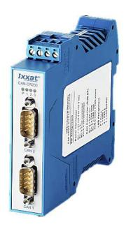
The Ixxat CAN-CR200 repeater with two CAN interfaces and one CAN backbone interface improves the CAN bus load capacity, establishes a physical coupling of bus systems and offers galvanic isolation. Multiple repeaters can be lined up and connected easily via the integrated DINrail bus to create various topologies and optimize network structures.
