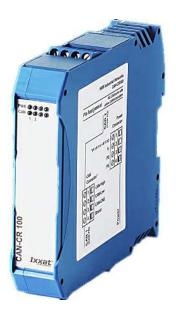
The Ixxat CAN-CR100 repeater with two CAN/CAN FD interfaces improves the CAN bus load capacity, establishes a physical coupling of bus systems and offers galvanic isolation. It provides the flexibility to optimize network structures and liberates them from CAN bus structure constraints for optimized operation.
