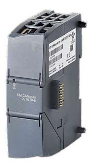
The Ixxat CM CANopen is a compact interface module designed for the integration of CANopen or CAN 2.0A devices with SIMATIC S7-1200 PLCs. Acting as a bridge with comprehensive support for CAN protocols, it facilitates communication and data transmission between devices and the PLC. For more flexible development and expansion of automation systems.
