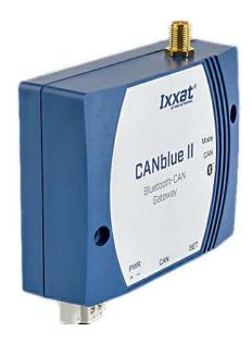
The Ixxat CANblue II is a versatile and cost-effective Bluetooth module for CAN systems that can be used with an external antenna. It offers three operation modes: PC interface, bridge, and gateway, making it suitable for various application areas. It is ideal for mobile configuration, analysis, and conveniently bridging CAN networks via Bluetooth.
