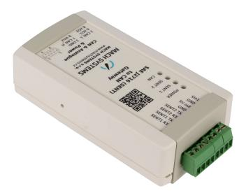
The SAE J2716 (SENT) to RS-232/CAN bus gateway features two bi-directional SENT (Single Edge Nibble Transmission) channels, two analogue output channels, and either RS-232 or CAN bus interface. The flexibility of the device allows the user to use it as a PC interface / SENT data logger, a gateway for PLC or a test system, and generally for SENT communication monitoring and simulation. The analogue outputs offer the possibility to directly convert SENT data frame signals into an analogue voltage.
