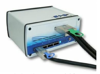
Access to the targets can take place with up to **100 MHz clock frequency** optionally via various serial interfaces such as **JTAG**, **cJTAG**, Device Access Port (**DAP/DAP2**) or Serial Wire Debug (**SWD**). Synchronization during debugging of several core/targets is achieved by the UAD3+ hardware and firmware. Two different input voltage ranges - **1.6 to 5.5 Volts** as standard or **optionally 0.8 to 3.3 Volts** - cover all possible applications.
