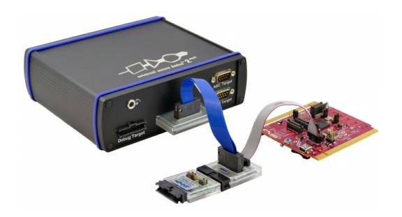
The UAD2<sup>next</sup> acts as a bridge between the base model UAD2<sup>pro</sup> and the high-end tool UAD3+. Besides a large number of powerful debug and trace interfaces, such as DAP, SWD, JTAG, cJTAG and LPD, the UAD2next also supports CAN and ASC interfaces for access to the target. Robust trace modules, which can be easily plugged in as needed, ensure a fast and efficient transfer of trace data from the target into the UAD2<sup>next</sup>.
