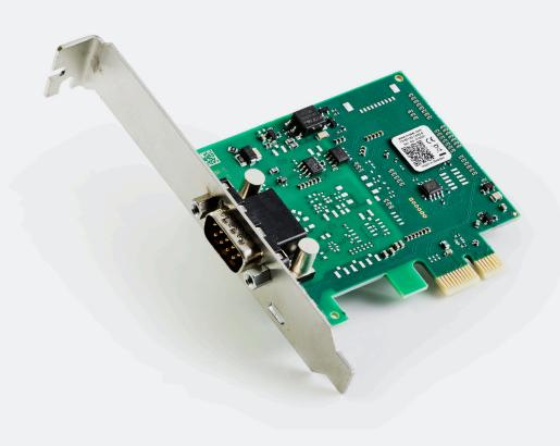
Kvaser PCIEcan 1xCAN v3 is a small, yet advanced, real time CAN interface that handles transmission and reception of standard and extended CAN messages on the bus with a high timestamp precision. The Kvaser PCIEcan 1xCAN v3 is compatible with applications that use Kvaser's CANlib.
