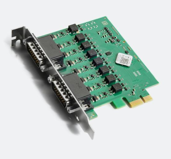
The Kvaser PCIe 8xCAN maximizes channel density through a single PCIe x1 slot, enabling the effortless design of advanced CAN systems.
