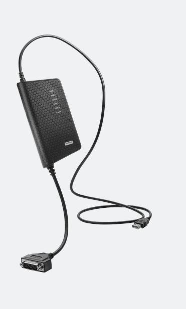
Kvaser USBcan Pro 5xCAN is a small, yet advanced, portable multi channel CAN to USB real time interface that handles transmission and reception of Classic CAN and CAN FD messages on the CAN bus with a high timestamp precision. The Kvaser USBcan Pro 5xCAN is compatible with applications that use Kvaser's CANlib.
