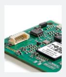
The USBcan Pro 2xHS v2 CB is a bare circuit board version of Kvaser's USBcan Pro 2xHS v2 dual channel CAN or CAN FD interface with scripting capability, the USBcan Pro 2xHS v2 CB is supplied 'bare board' i.e. without a housing, and can thus be built into any system.
