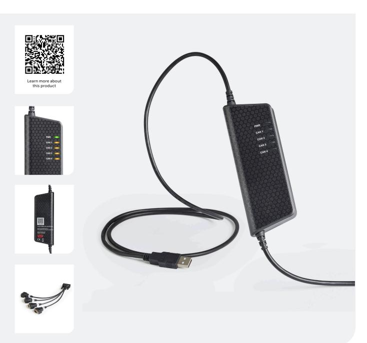
The USBcan Pro 4xCAN Silent, a compact, multichannel four-channel CAN/CAN FD to USB real-time interface that is always silent on the CAN bus ('listen only'). This CAN interface is made silent through hardware and thus, cannot transmit on bus.
