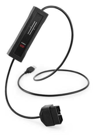
The Kvaser U100-X3 is a robust, galvanically-reinforced single-channel CAN/CAN FD to USB interface with a 16-pin OBDII plug.
