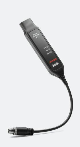
Kvaser Air Bridge M12 is a small, yet advanced, wireless CAN bridge that can be used to form a CAN system bridge, when paired with any other Kvaser Air Bridge M12 device and create connectivity between two or more CAN networks. This radio solution can be used to connect CAN based control systems and test equipment in scenarios and situations where it is desirable to replace cabling and related parts.
