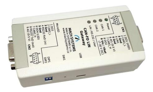
**The CAN-FD LIN Gateway** is a user-programmable converter/router/data-logger that features two CAN FD channels, a LIN channel, and a RS-232 port. The converter offers a microSD card slot and multiple digital/analogue inputs and outputs, and its firmware can be developed in C or C++. The device is suitable for a broad range of applications such as protocol conversion, network bridging, data logging, rest-bus simulation, and external peripheral control and monitoring.
