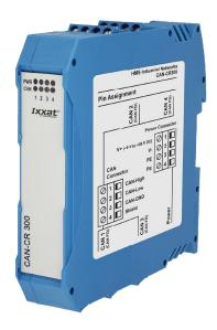
The CAN-CR300 is used for galvanic isolation of CAN / CAN FD network segments and to design tree or star topologies. As a special feature, the repeater separates a defective segment from the rest of the network, allowing the remaining network to continue working. After the fault has been eliminated, the segment is automatically switched back to the network. The galvanic isolation is provided for the CAN / CAN FD segments as well as for the power supply.
