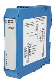
The CAN-CR120/HV is used for galvanic isolation of two segments of a CAN / CAN FD network. As a special feature, the repeater separates a defective segment from the rest of the network, allowing the remaining network to continue working. After the fault has been eliminated, the segment is automatically switched back to the network. The galvanic isolation is provided for the CAN / CAN FD segments as well as for the power supply.
