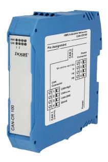
The CAN-CR100 is used for galvanic isolation of two segments of a CAN / CAN FD network. As a special feature, the repeater separates a defective segment from the rest of the network, allowing the remaining network to continue working. After the fault has been eliminated, the segment is automatically switched back to the network. The galvanic isolation is provided for the CAN / CAN FD segments as well as for the power supply.
