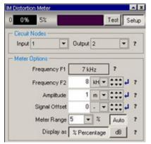
The CCIF test uses a source made up of two high frequency, equal amplitude components whose frequencies are separated by a small frequency (e.g. 1Kh). The program defaults to source signal components at frequencies of 13kHz and 14kHz. With this test, the percent intermodulation distortion is defined as the amplitude of the frequency component at Fh-Fl as a percentage of the source amplitude.
