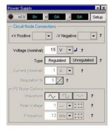
The power supply noise's frequency equals twice the wall voltage's frequency, for example, 120 Hz, when the wall voltage is at 60 Hz. The noise's waveform is selectable. Actual capacitor smoothed power supplies produce a triangular noise waveform; choke input power supplies, something closer to a sine wave waveform; and some switching power supplies, a square wave waveform.
