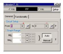
The meter displays its voltage measurements in two ways: text and a moving bar graph.
