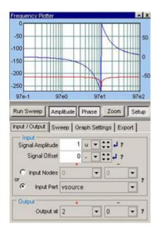
The last tab, Export, allows you to export the graph to various formats, including graphic files, text tables, or even copy it to the Project's graph window. You can even copy the graph into memory to paste into other applications. Pressing the "Zoom" button brings up a new window with just the graph portion of the small frequency sweep instrument.
