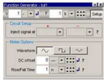
Pressing the "Setup" button toggles the height of the Function Generator, so that when its setup is complete, the it becomes only as tall as its display band.
